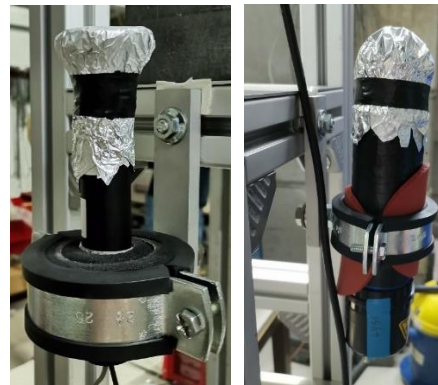
Fig. 3: 1'' PMT (left) and 2'' PMT (right) configurations
